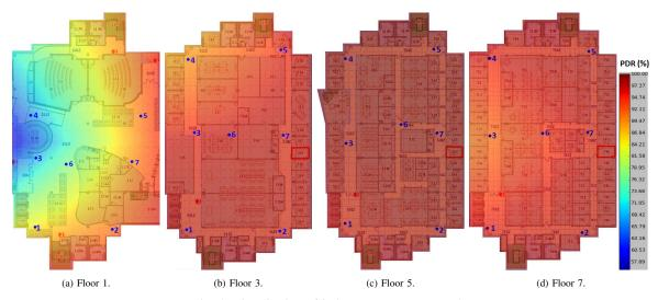
Fig. 4: Visualization of indoor measurement results.
