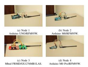
Fig. 3: Custom-built LoRa end devices.
