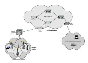
Fig. 1. All-IP wireless network architecture
