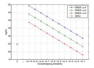
Fig. 6: Power consumption of SERJ and SMER versus eavesdropping probability for various values of  $\alpha$  and when  $n_E=5$  eavesdroppers are present. For small secrecy outage probabilities, the power consumption of SMER is substantially higher than the power consumption of SERJ.
