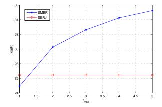
Fig. 11: Power consumption of SERJ and SMER versus the uncertainty in the location of the eavesdropper (i.e.  $r_{max}$  around each transmitter in the network). The transmit power using SERJ is independent of the location of the eavesdroppers. But with SMER, as the uncertainty in the location of the eavesdroppers increases the power consumption increases.
