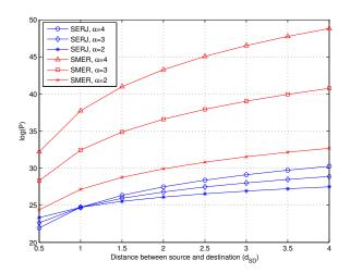
Fig. 7: Power consumption of SERJ and SMER versus the distance between source and destination  $d_{SD}$  for various values of  $\alpha$  and when  $n_E=5$  eavesdroppers are present. As the distance between the transmitter and the receiver gets longer, the transmit power of both schemes increases.
