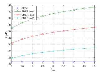
Fig. 5: Power consumption of SERJ and SMER versus  $r_{max}$  for various values of  $\alpha$  and when  $n_E=5$  eavesdroppers are present. The performance of SMER is closely dependent on the uncertainty in the locations of the eavesdroppers, while the performance of SERJ does not depend on the locations of the eavedroppers.
