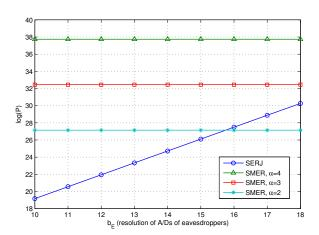
Fig. 8: Power consumption of SERJ and SMER versus the resolution of eavesdroppers' A/Ds  $b_E$  for various values of  $\alpha$  and when  $n_E=5$  eavesdroppers are present. As  $b_E$  become higher, with SERJ we need more jamming power and thus the power consumption of SERJ increases while with SMER, the performance is independent of the quality of eavesdroppers' A/Ds.
