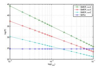
Fig. 4: Power consumption of SERJ and SMER versus the radious  $r_{min}$  of the guard region for various values of  $\alpha$  and when only one eavesdropper is present. As we allow the eavesdropper to become closer to the transmitter (i.e. as  $r_{min}$  gets smaller), the power needed to make the link secure using SMER becomes higher. On the other hand, with SERJ there is no need to assume a guard region around the transmitter.
