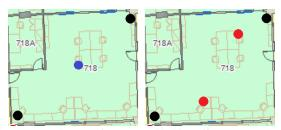
Fig. 1: Scenario 1: Two clients in a 10x10m office space. In Mode-1 (left) there is 1 beamforming AP in the middle, and in Mode-2 (right) there are 2 omnidirectional APs. The black circles are WiFi clients.
