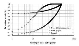
Fig. 3: Top 8 markers can represent from 10% to 70% off all bytes.
