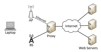
Fig. 5: Experimental Setup with the Remote Proxy.
