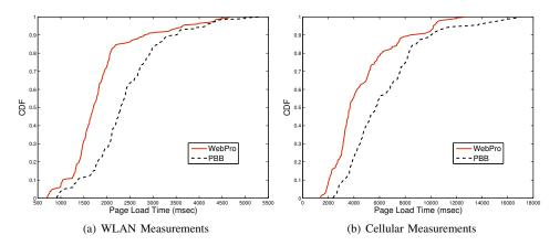
Fig. 7: Cumulative Distribution Function of Page Load Time. WebPro outperforms benchmark PBB. In the WLAN setting, under WebPro, 73% of the pages load in less than 2 seconds. However, in the PBB approach, 28% of the instances complete loading within 2 seconds. In the cellular environment, under WebPro, 78% of the page loads complete within 6 seconds while under PBB, only 55% of the pages complete loading in that time.
