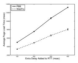
Fig. 10: Average Page Load Time for a Wikipedia article page as a function of network delay. We see that higher RTT values lead to higher page load times. By increasing RTT, PBB incurs higher latencies compared to WebPro.
