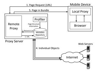
Fig. 3: High Level Architecture of WebPro.
