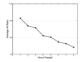
Fig. 6: Temporal Change in Webpage Structures. Drop in the value of the average hit ratio over time is an indication of the change in the structure of the webpages. However, the amount of such change is relatively low over an eight hour period.
