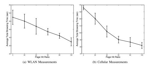
Fig. 8: Back to Back load time for 20 popular webpages as a function of page hit ratio. An increase in the page hit ratio reduces the total browsing time. In the case of WLAN and cellular measurements, there is a maximum reduction of 28% and 39%, respectively. The maximum improvements are achieved at 100% page hit ratio.
