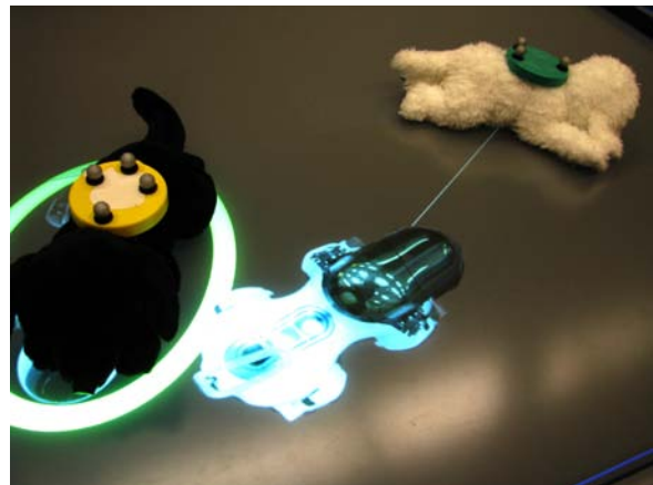
(c) The TUI interface. The green halo around the black dog means the black AIBO has reached its target. The white AIBO icon represents the physical robot's location, attempting to follow the line toward the target location defined by the white-dog toy.
