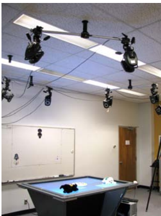
(a) The tabletop workspace with the TUIs on top and the Vicon ceiling setup.
