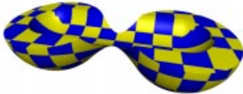
Figure 10: Texture space discontinuity across a CSG intersection.
