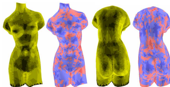
Figure 4: Shaded relief images of Venus model (5,584 faces) with (1) lighter yellow referring to greater slope steepness, and with (2) darker blue and red referring to regions of greater convexity and concavity, respectively.
